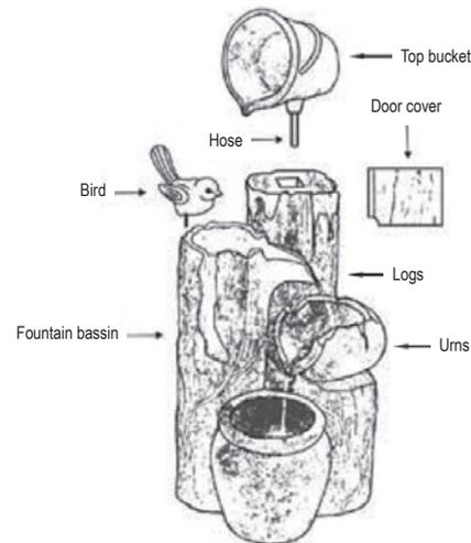
5.2 Attach pump to the hose from access panel on rear of logs. LED light is pre-assembled in lower urn. The pump and LED light cables exit out from rear access panel, ready for connection to solar panel.
