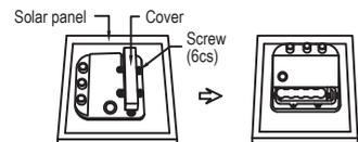
8.3 Disconnect the connectors, then replace the old battery pack with a new battery pack and join the connectors together
